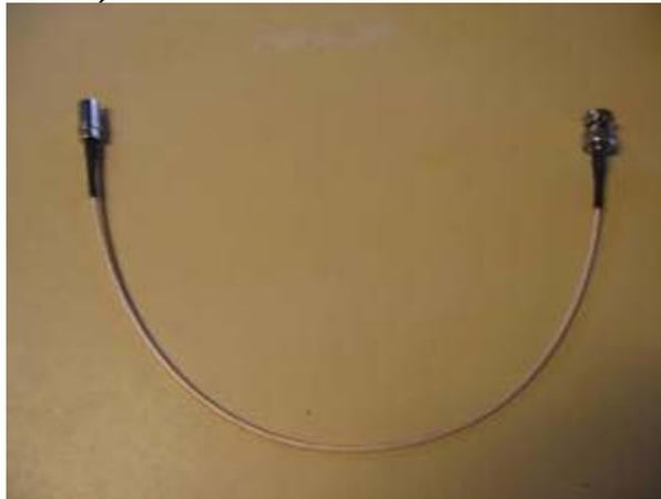
Attach one end of this coax matching section to the Feed Point described above.
