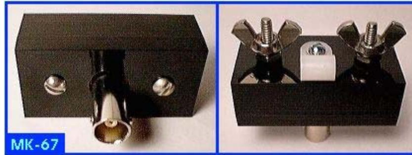
(See [Figure 2](#).) There is no up or down on the connector, so you can attach either end of the loop wire to either one of the wing nuts.
