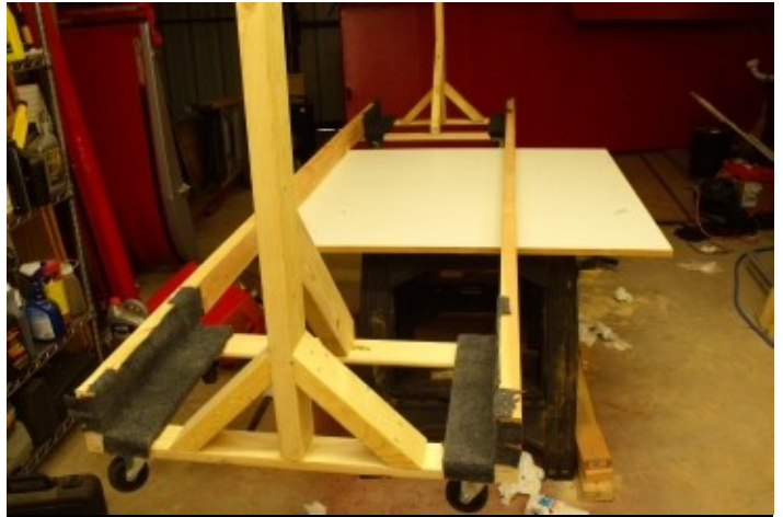
The complete wing dolly ready to cover with padding
