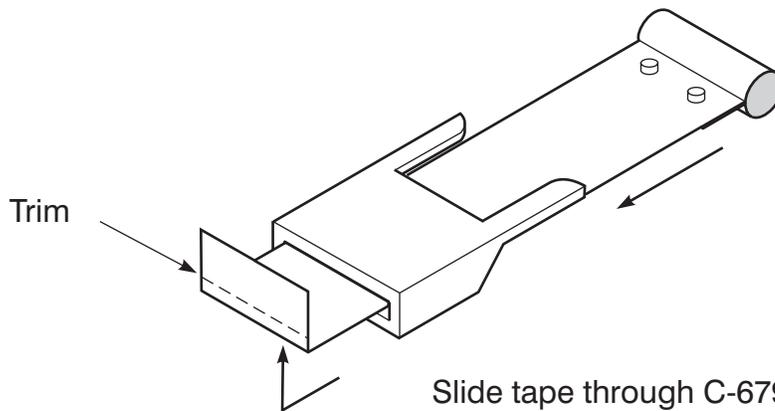
Slide tape through C-679 (make sure part is right-side up) and bend end of tape up at desired length for lanyard. Trim end so that C-679 will be retained but end of tape will not contact canopy skirt in closed position
