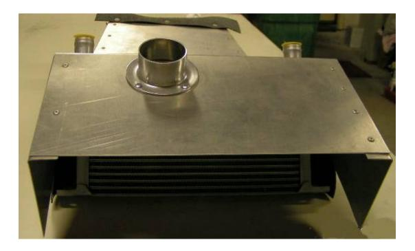
The two plenum chambers are made from aluminum chassis boxes (normally used for electronic projects). These are available in a variety of sizes and shapes from various electronics supply shops. Here I have used a small box for the warm air plenum and a larger one for the mixing plenum primarily to get things to fit. My original scheme was to use a single box but because I designed the system after too many other things were in place I did not have room for a single plenum.
